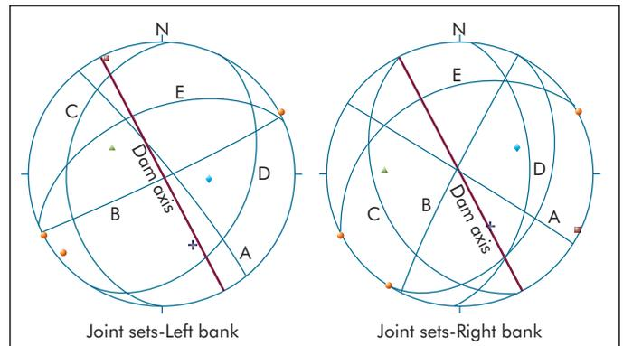
Figure 2 – Stereographic projection of the five joint sets for the left and right banks, with dam axis
