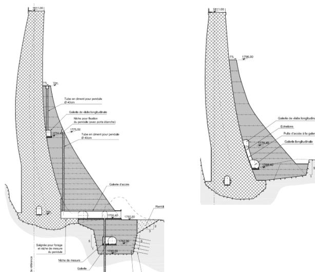
Figure 3: Cross-sections of existing dam and reinforcement;
