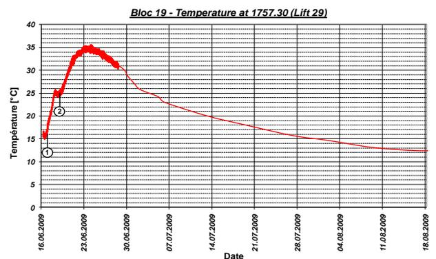
Figure 8: Concrete temperature vs. time curve showing temperature rise caused by cement hydration heat and subsequent effect of post-cooling
