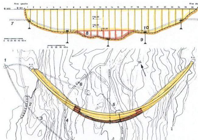
Figure 1: Existing dam upstream face and layout
